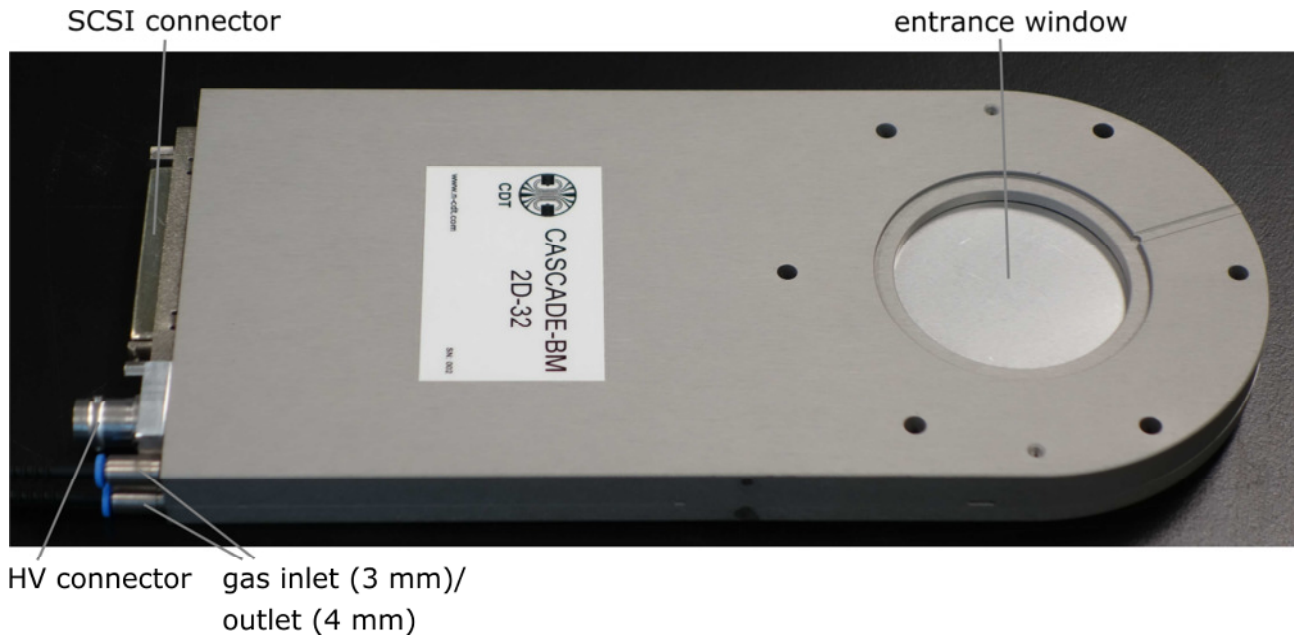
Picture of the CASCADE-BM 2D-32 detector housing: neutron entrance window made of 100 \mu\text{m} Aluminum (right side), gas inlet and outlet as well as HV connector of type SHV and SCSI-III connector for the DAQ electronic readout and powering (left side).
