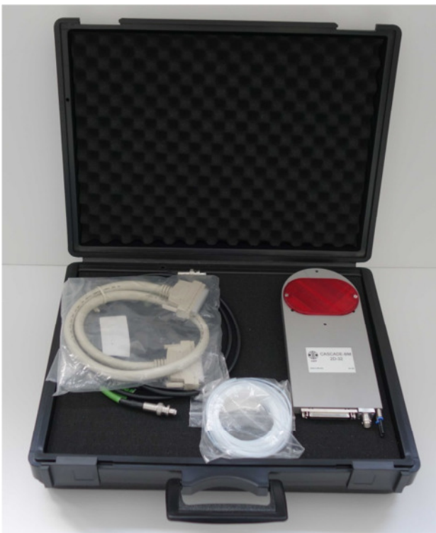
CASCADE-BM 2D-32 beam monitor detector system. The detector itself is shown on the right side with a transport secure shield (red) for the very thin entrance window. Gas supply pipes, a high voltage cable and a SCSI-III data cable are shown as well.
